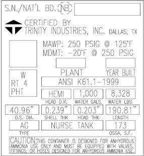
**ASME** Nameplate Requirements: Required nameplate markings per the ASME Code, Section VIII, Division 1, UG-116 through UG-119 for the years after 1988 Addendum.
