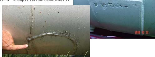
(4) 49 CFR Section 173.24(b)(2) – Tanks used for the shipment of anhydrous ammonia must be properly maintained. A reduction in package (or tank) integrity poses an unsafe and increased risk of failure during conditions normally incident to transportation (vibration, shock, and loading). Many tanks were observed
